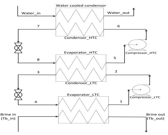
Figure 1: Two stage vapour compression cascade refrigeration system using HFO refrigerants
