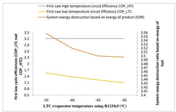
Figure 14 : Variation of system exergy destruction ratio based on exergy of product(EDR\_System) and cycle coefficient of performance (Cycle First law efficiency ) of HTC and LTC with temperature of low temperature evaporator
