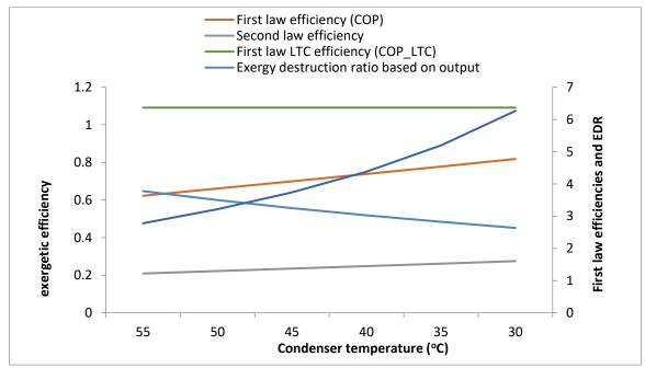
Figure 2 :Variation of First law efficiency (Coefficient of performance: COP\_Overall) and second law efficiency (exergetic efficiency), Exergy Destruction Ratio based on exergy of product HTC first law efficiency (COP\_HTC) and LTC first law efficiency (COP\_LTC) with condenser temperature(°C)
