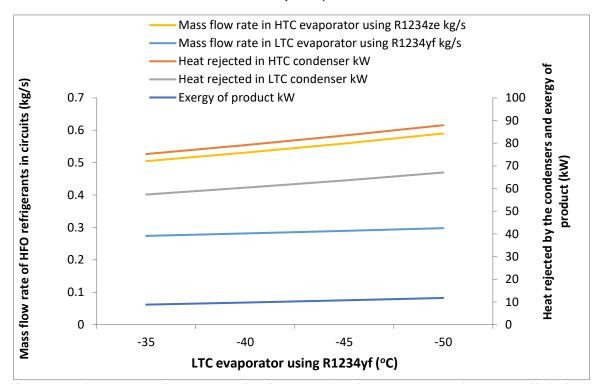
Figure 16 : Variation of system exergy destruction ratio based on exergy of product ( $EDR_{System}$ ) and Heat rejected by high temperature condenser (kW) ) using R-1234ze and Heat rejected by cascade condenser (kW) using R-1234yf with Low temperature evaporator ( $^{\circ}C$ )
