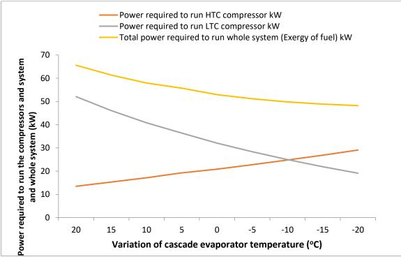
Figure 11:Variation of power required to run the system/ exergy of fuel (kW), power required to run high temperature compressor (kW) using R1234ze , power required to run low temperature compressor (kW) using R1234yf with temperature of cascade evaporator temperature ( $^{\circ}C$ )
