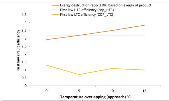
Figure 6: Variation of High temperature circuit first law efficiency in terms of Coefficient of performance (COP\_HTC), Low temperature circuit first law efficiency of system in terms of Coefficient of performance (COP\_LTC), and exergy destruction ratio based on exergy of product (EDR\_System) with temperature overlapping (°C) in cascade system
