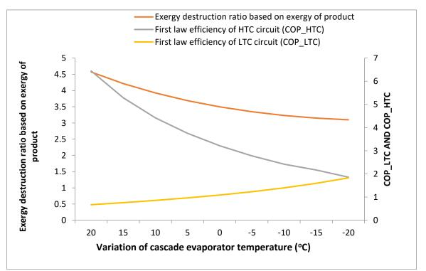
Figure 10: Variation of HTC first law efficiency (COP\_HTC) and HTC first law efficiency (COP\_LTC) and exergy destruction ratio based on exergy of product with temperature of cascade evaporator temperature (°C)
