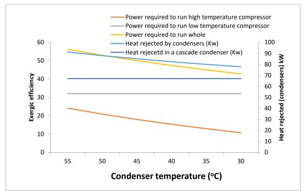
Figure 3 :Variation of heat rejected by high temperature condenser (kW), heat rejected by cascade condenser (kW), total power required to run whole system (Exergy of fuel) kW and power required to run HTC Compressor using HFO R1234ze (kW), power required to run LTC Compressor using HFO R1234yf (kW) with condenser temperature(°C)
